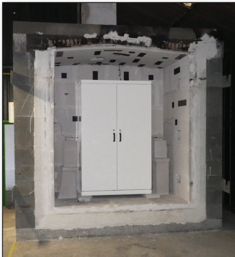
^795 cabinet placed into the oven to fire test according to EN 14470-1 norm (photography before test).
