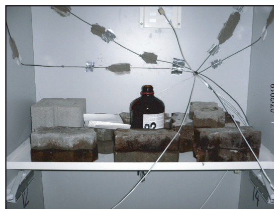
^ Sensors in a flammable cabinet
