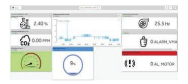
The system has a difference of less than one minute in displaying data, but the system is independent of the building's computer network, allows multi-user access in a decentralised manner and the cost of expanding new equipment is much lower than that of a SCADA.
